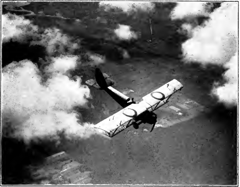
Fig. 10 —Since an Airplane is a very small object when viewed at a few thousand feet, any pattern used to render it of low visibility should obviously cover a large portion of the wing surface.
